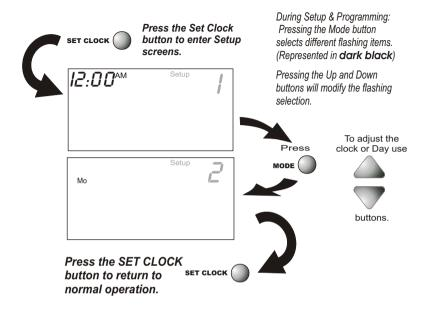
The thermostat is preprogrammed from the factory to operate 1 stage of cooling or 2 Stages of heating equipment\* without the need for further programming. To optimize the installation of this thermostat follow the instructions in the Advanced Setup section.
